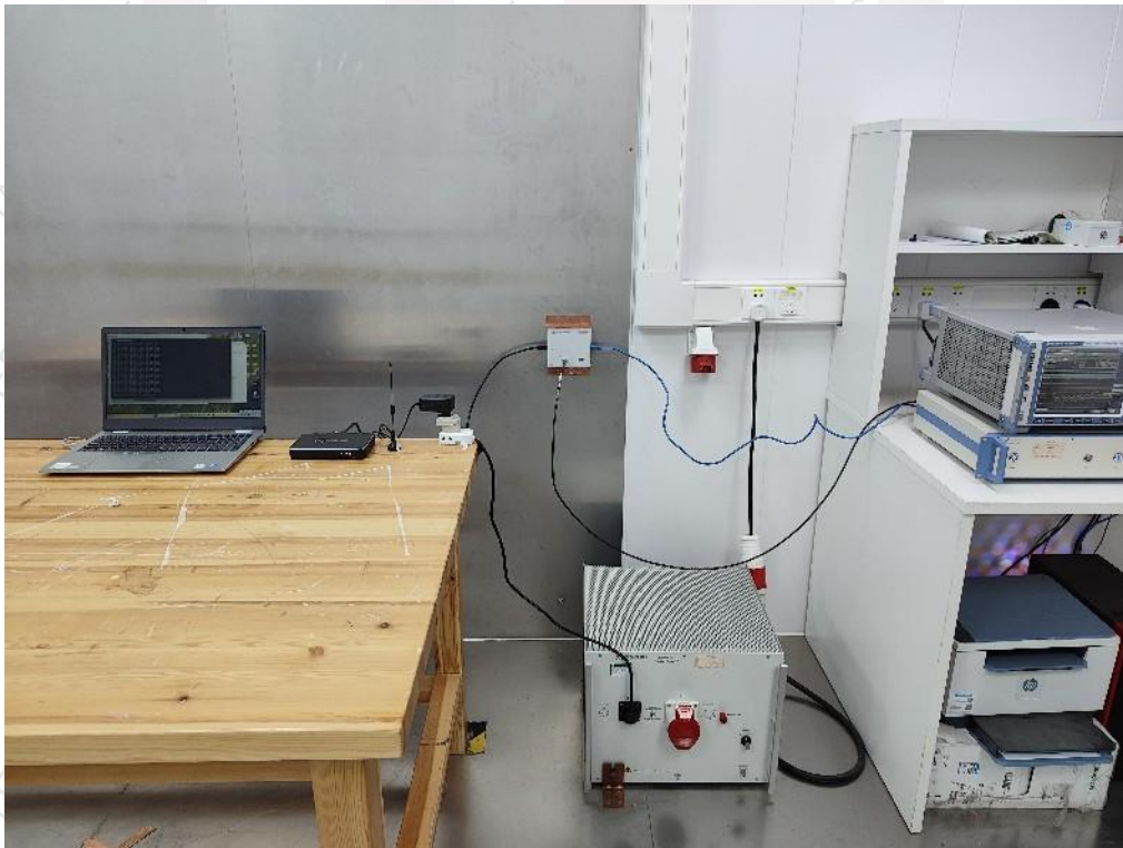
Photographs 2: Set-up for Asymmetric mode conducted emission
