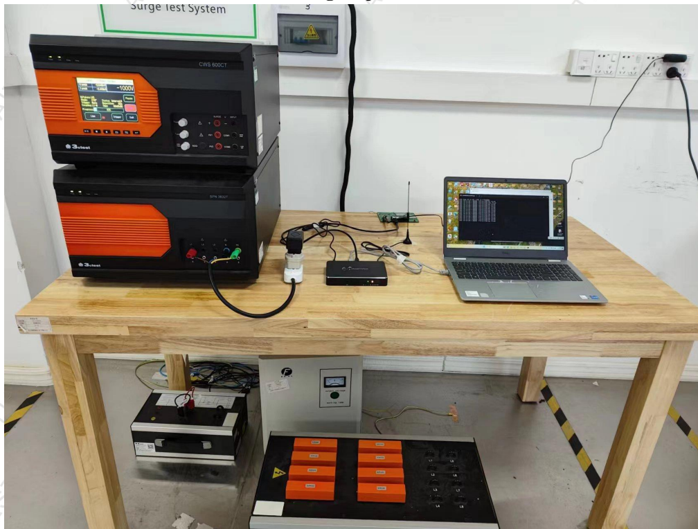
Photograph 10: Set-up for Conducted disturbances, induced by radio-frequency fields (CS)
