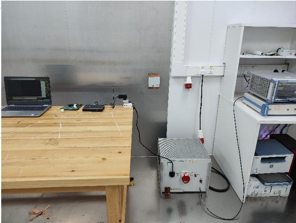
Photographs 2: Set-up for Asymmetric mode conducted emission
