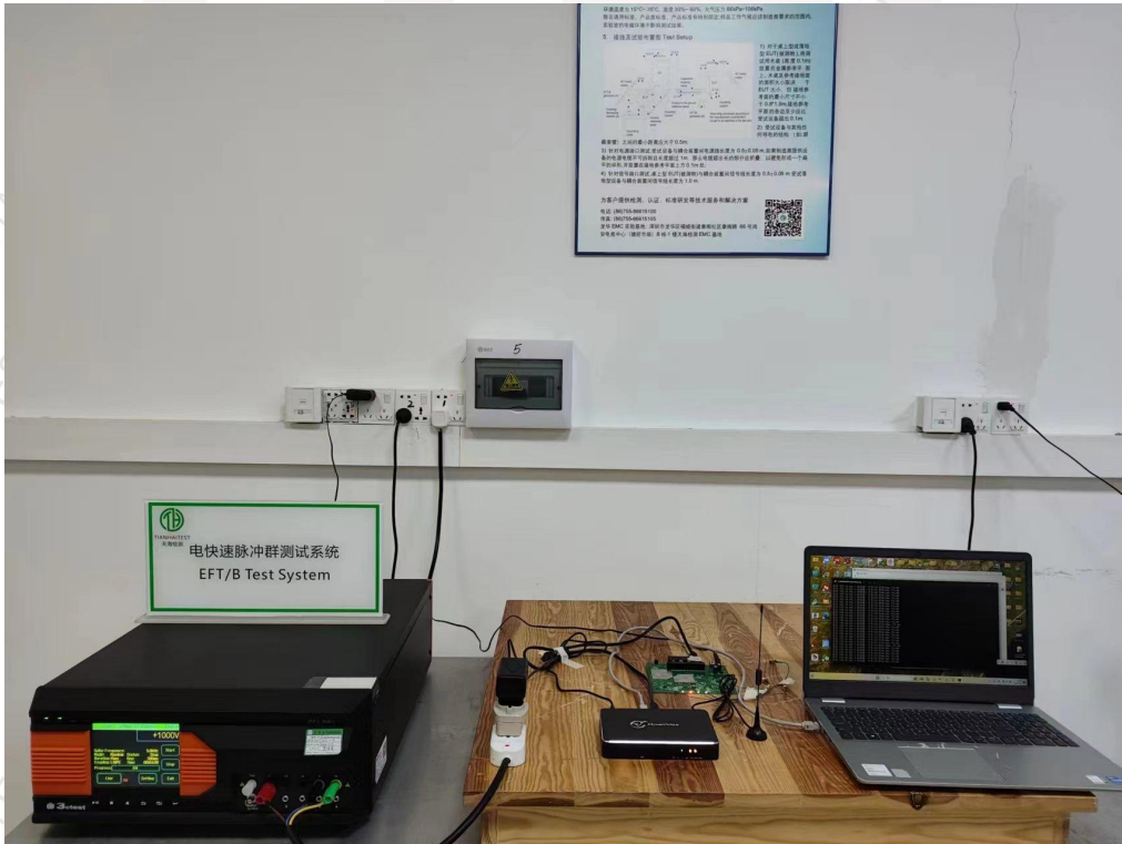
Photograph 8: Set-up for Electrical Fast Transient / Burst(EFT) AC power port
