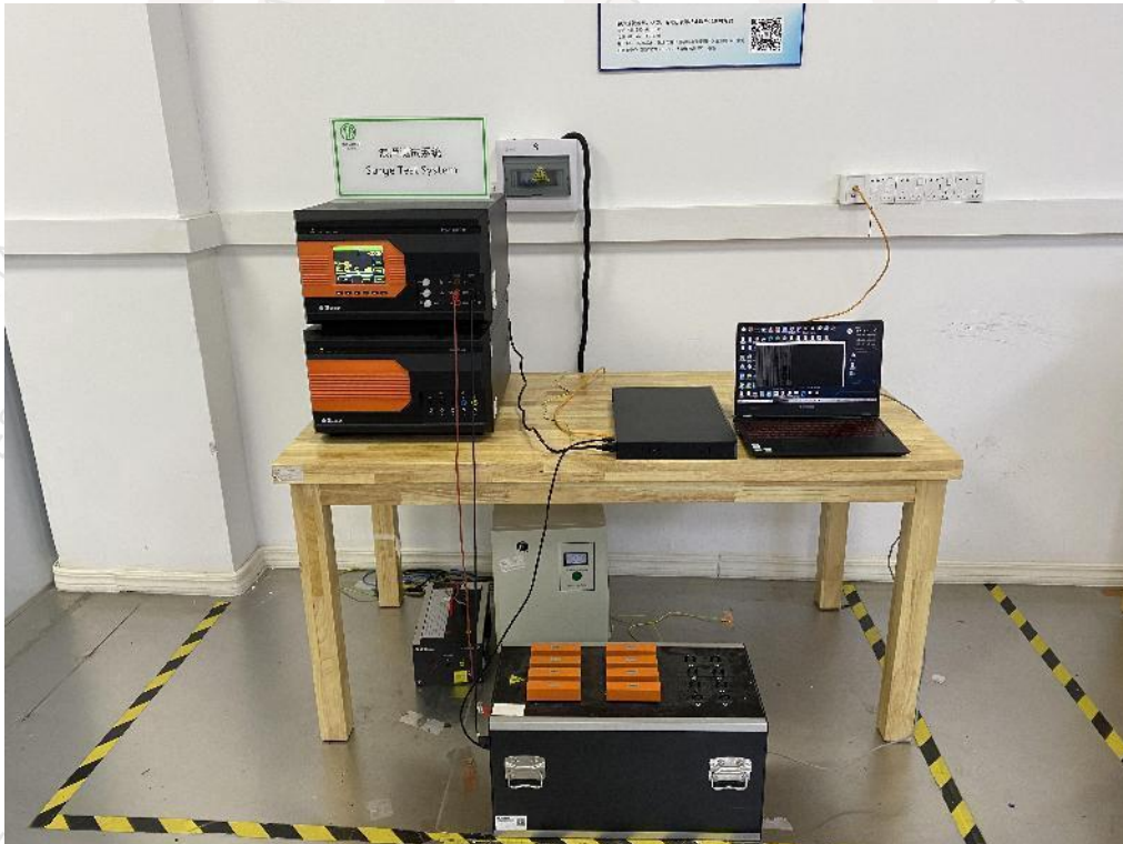
Photographs 10: Set-up for Surge -Signal port
