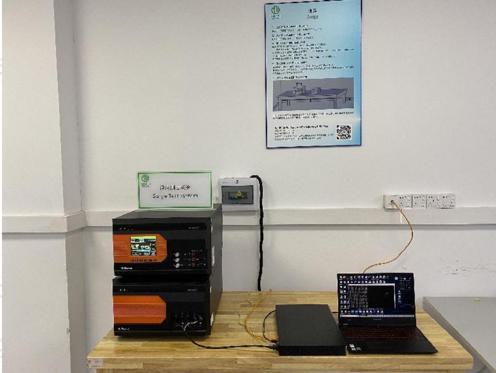
Photographs 9: Set-up for Surge -AC power port
