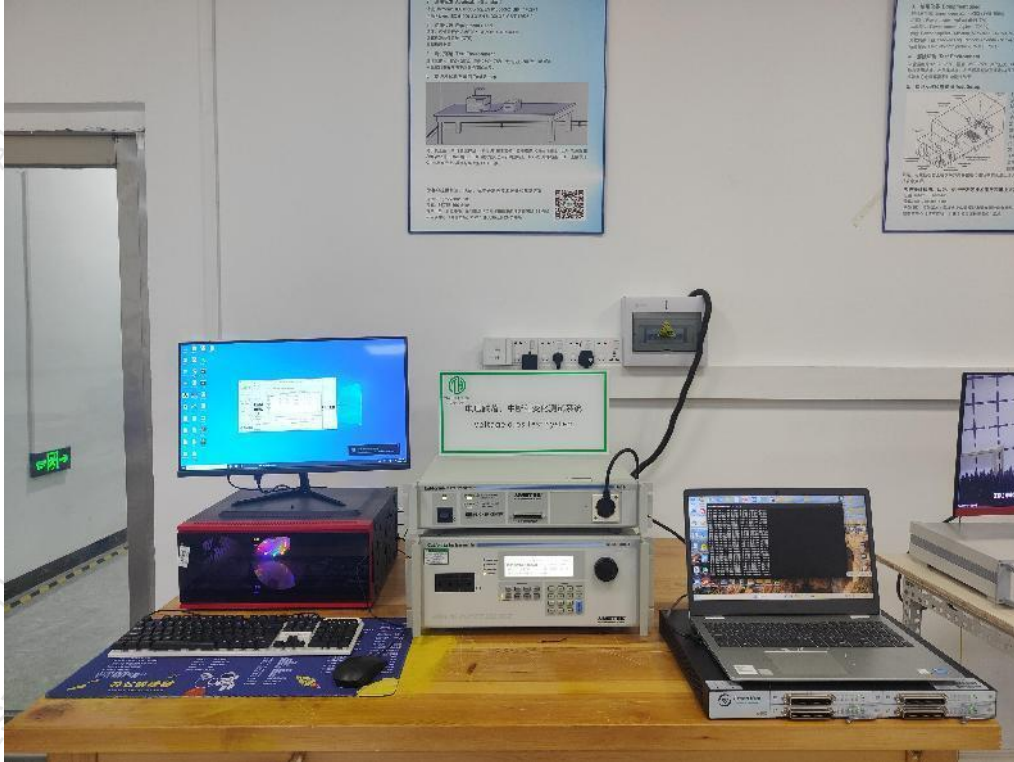
Photographs 13: Set-up for Voltage dips & Voltage interruptions
