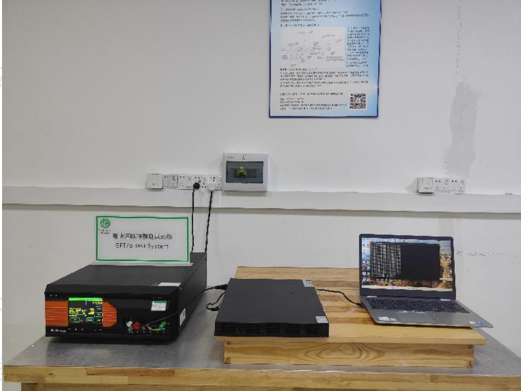
Photographs 7: Set-up for Electrical fast transient (EFT)-AC power port
