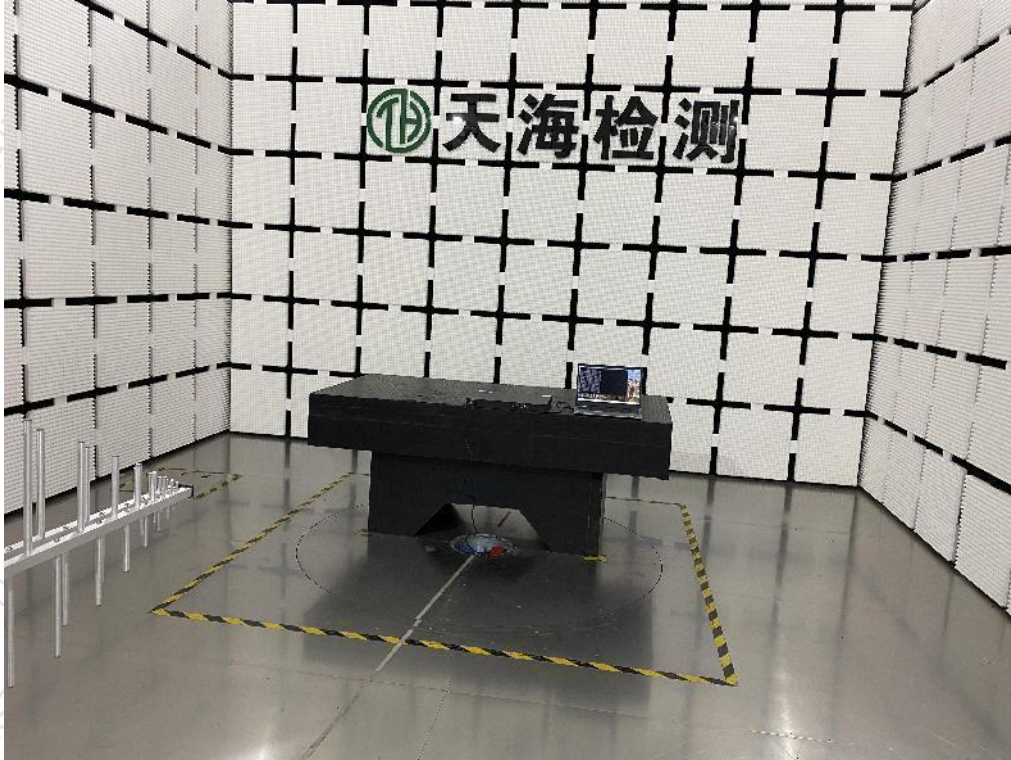
Photographs 3: Set-up for Radiated disturbance(below 1GHz)
