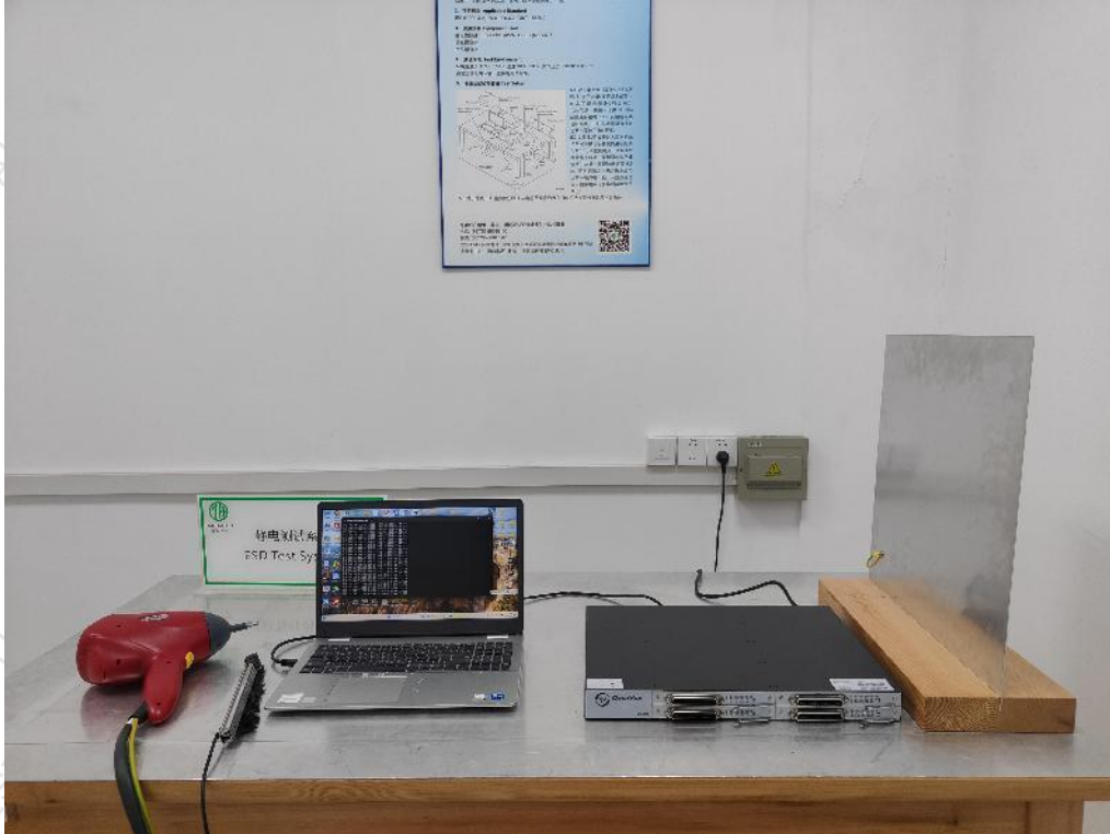
Photographs 5: Set-up for Electrostatic discharge (ESD)
