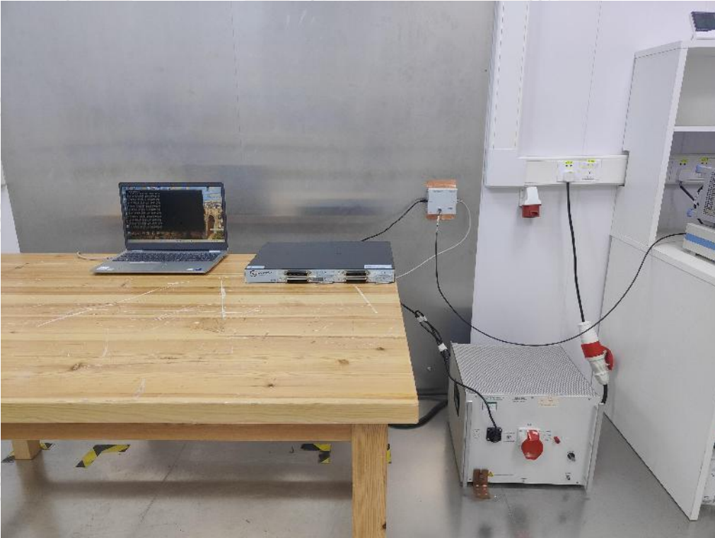
Photographs 2: Set-up for Asymmetric mode conducted emission
