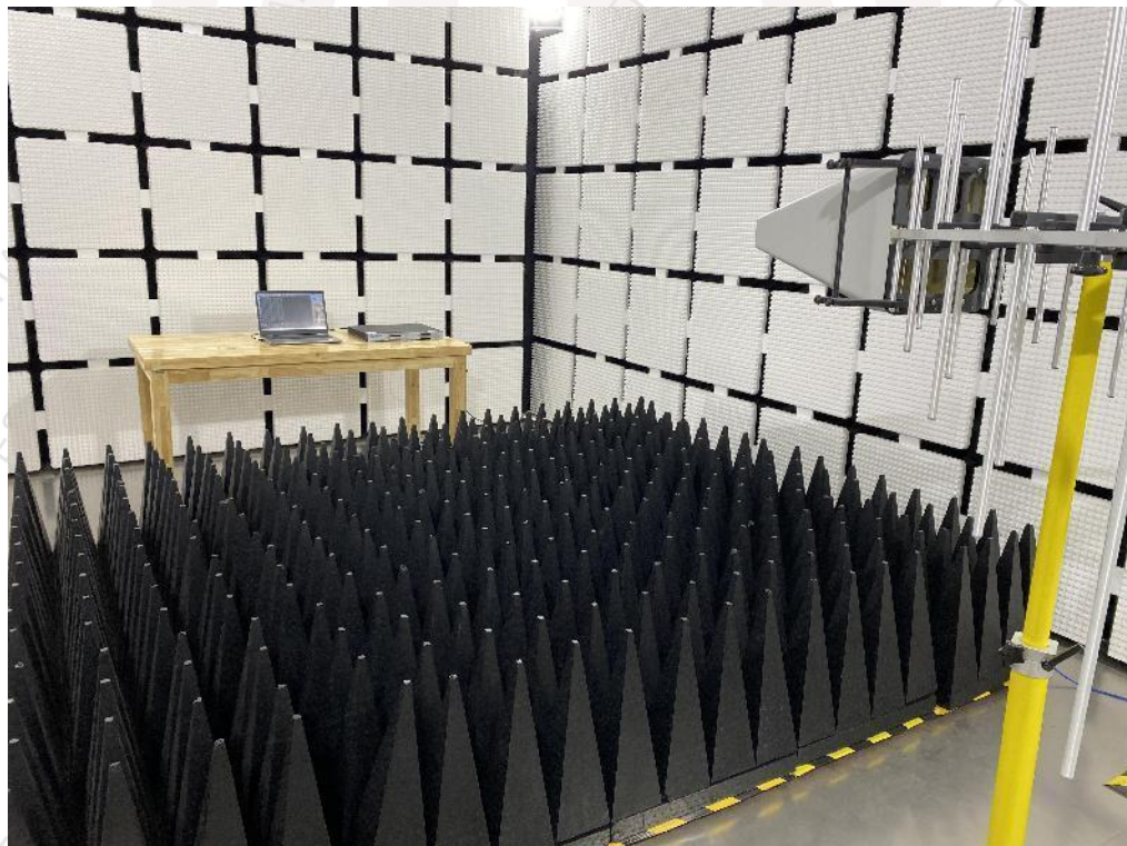
Photographs 6: Set-up for Radio-frequency, Continuous radiated disturbance(RS)
