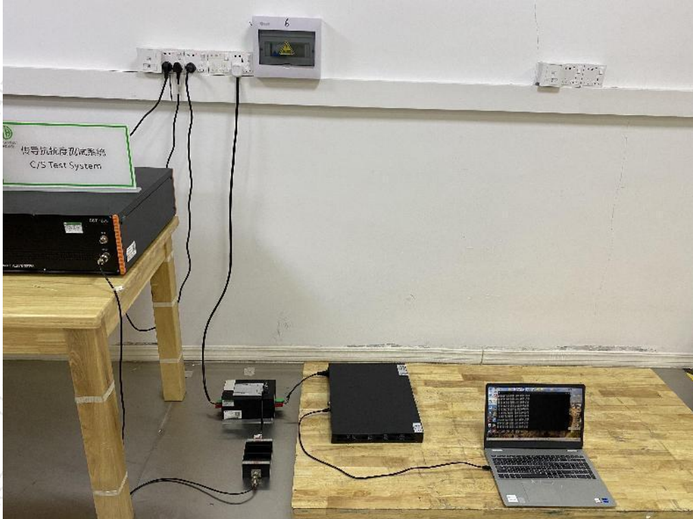
Photographs 11: Set-up for Radio-frequency, Continuous conducted disturbance (CS)-AC power port
