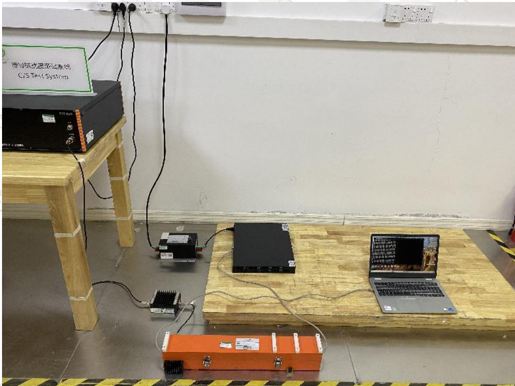
Photographs 12: Set-up for Radio-frequency, Continuous conducted disturbance (CS)-Signal port
