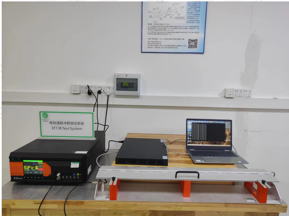
Photographs 8: Set-up for Electrical fast transient (EFT)-Signal port
